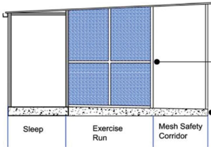
Division walls between units to have either solid or opaque panels – not clear glass or open mesh
